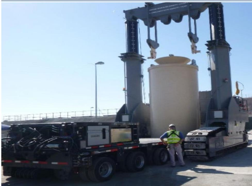
15 A vertical cask transporter is used to move the transfer cask into position on the
