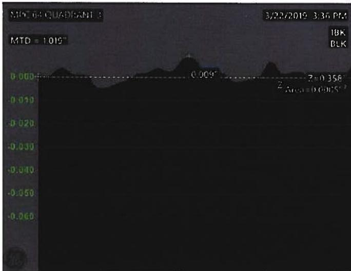
The figures above correspond to the shield ring induced wear marks identified between MPC Inner Seismic Restraints 5 and 6 as documented in Table 1 in the body of the report.
