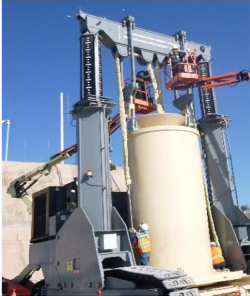
This photo shows the canister ready for downloading, the vertical cask transporter lift beam has been raised, and the full load of the spent fuel canister is being suspended. The mating device door is open, allowing the canister to be downloaded into the ISFSI vault. (Ex. 4, p. 7)
